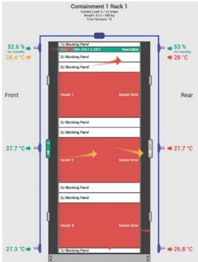
Cabinet rack map displaying thermal maps in AKCPro Server
